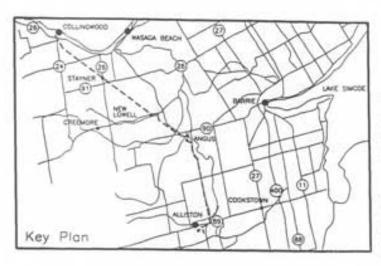
The pipeline is 57 km long and starts at the Raglan Water Plant in Collingwood and terminates at the Parson's Road Reservoir in Alliston.
